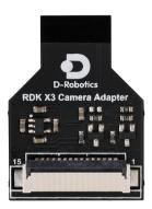
RDK X3 Camera Adapter is designed for compatibility with the D-Robotics RDK X3 platform. It converts the native CSI interface of the RDK X3 into a 15-pin, 2-lane CSI interface, enabling seamless integration with popular Raspberry Pi-compatible camera modules such as the OV5647, IMX219, and IMX477.
