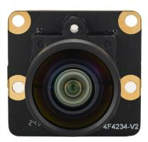
The RS400W HD camera module is specially optimized for the RDK X3 platform, featuring a compact design with high sensitivity and low noise for excellent imaging performance. It connects directly via a standard CSI interface and supports up to 2560×1440 resolution at 60 FPS, making it an ideal solution for robotic vision, industrial inspection, and other applications.
