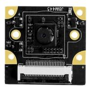
The RS800W dedicated HD camera module features a compact design and is equipped with a high-sensitivity sensor. It delivers high-speed and stable image transmission through the CSI interface, providing a professional-grade imaging solution for Al vision applications such as industrial inspection and robotic navigation.
