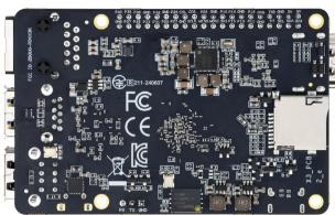
The D-Robotics RDK X3 is a next-generation high-performance intelligent platform specifically designed for AloT and robotics applications. It features D-Robotics's self-developed Sunrise® 3 series chip, delivering up to 5 TOPS of edge Al computing power and a quad-core ARM Cortex®-A53 processor. Combining low power consumption with high efficiency, it enables developers to quickly build intelligent applications.
