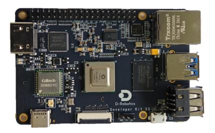
RDK X3 include a quad-core Cortex®-A53 processor, 5Tops BPU computational power, up to 4GB of RAM, and support for 4K@60fps video encoding and decoding. The primary interfaces include HDMI, Gigabit Ethernet, USB 3.0, USB2.0, MIPI CSI, UART Debug, and TF card slots.
