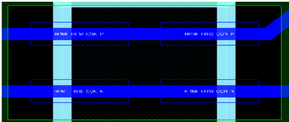
Figure 8-18. SMT Pad Trace Entering
