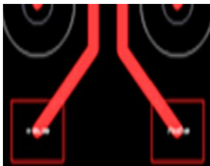
Figure 8-18. SMT Pad Trace Entering
